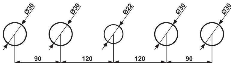
After preparing the tub body, insert the faucet components into the holes provided and secure with the appropriate nuts.
